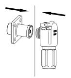
Note: Press the position indicated in the figure above before disconnecting the power terminal.
